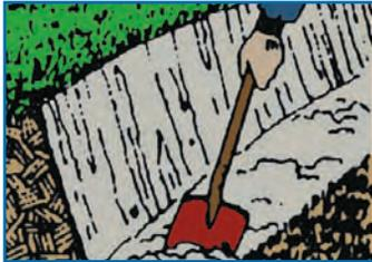
Excavate a trench approximately 14 inches wide. Follow this table for trench depth and thickness of the compactible rock leveling base.
